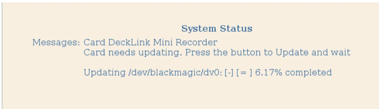
Do not power off your computer until this process ends, it could damage your card. Once you see the 100% completed message, you will be conducted to reboot your machine from the Network Tab. Once rebooted, the new driver will work properly with the new driver and you will see on Status a message with the name of the card detected by the driver, and of course “card successfully updated”. Now we can start to work with the encoder.
