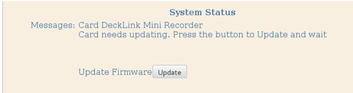
Here we have a very common situation, where the card has been detected or not, and needs a firmware update to work properly. When new BMD drivers are added or brand new cards are plugged in, this is a very common picture. So just connect your computer to the Internet and press Update. In seconds it will start to download the latest Firmware from BMD servers and will burn it on the ROM of the BMD PCIe card to work properly with the latest loaded drivers.
